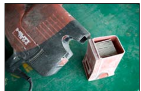
Drill with dust removal system
