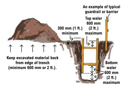
Vertical supports must extend above the ground level a minimum of 300 mm (1 ft.) and must be no more than 600 mm (2 ft.) up from the bottom of the trench.
