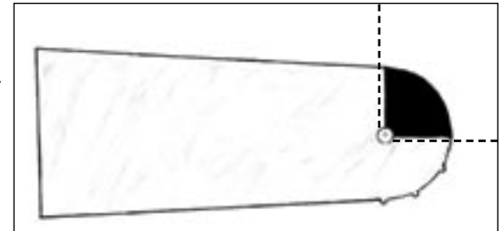
Make sure to avoid contact in the kickback zone (shown in black).
