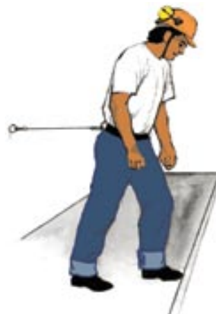
This is an example of a fall restraint system. Fall restraint systems prevent workers from falling.
